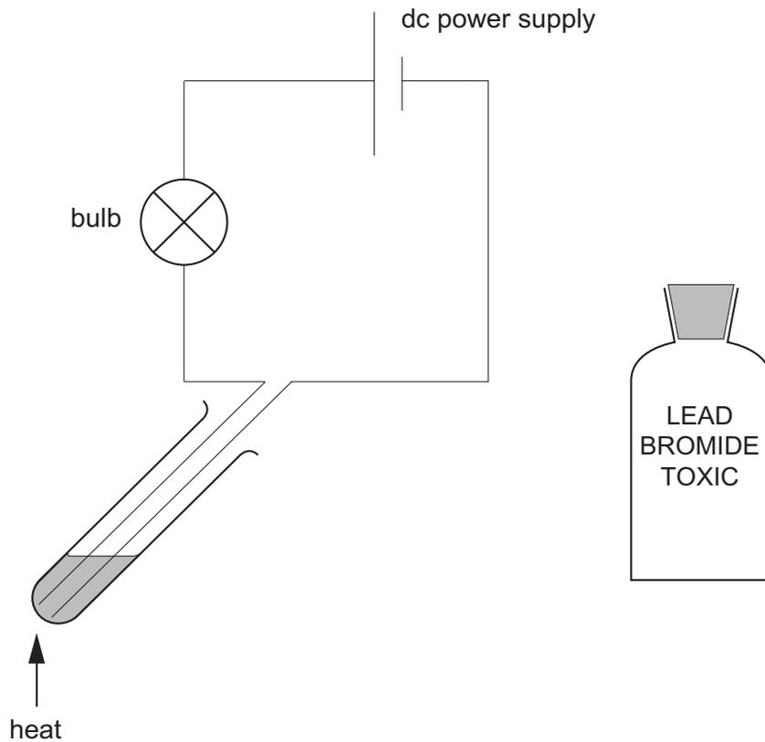
The lead bromide was heated until molten. A brown gas was given off.
